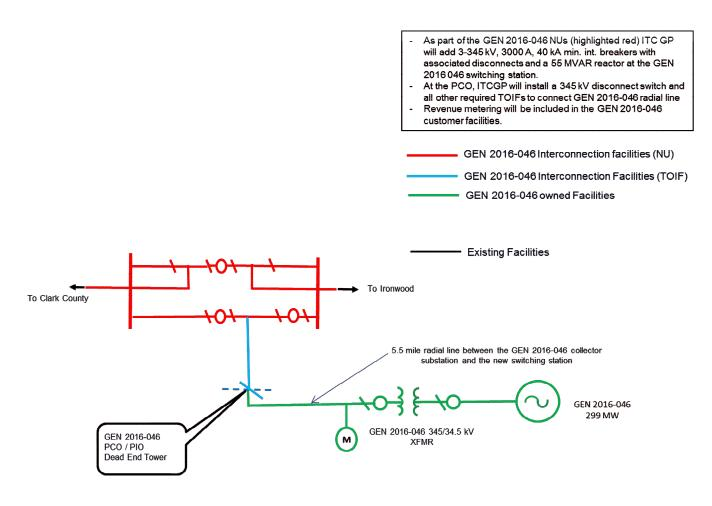
Figure 1 GEN-2016-046 ITCGP Interconnection Substation One Line
